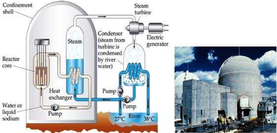
Basic design of a nuclear power plant. C(a) A fluid such as water or liquid sodium carries heat produced by the reactor core to a heat exchanger in which steam is generated. The heat exchange liquid moves in a closed loop. The steam is used to drive an electrical generator. (b) A nuclear power plant in New Jersey. Notice the dome-shaped concrete
